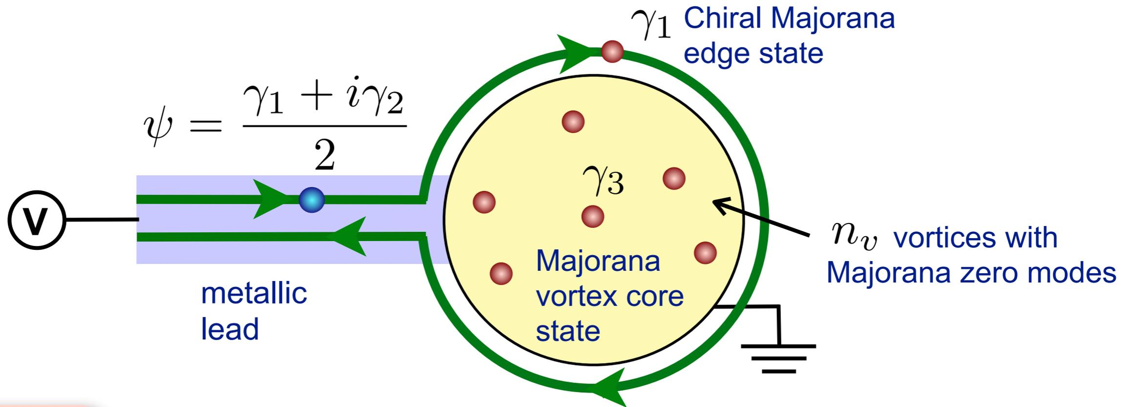
$n_v$  : odd **injected electron (hole) is perfectly converted to hole (electron) !! (perfect Andreev reflection)**
